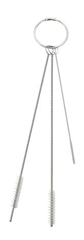
The brush set is suitable for cleaning very small nozzles and valves on eg. coffee and juice machines. The brush heads have a diameter of Ø2, Ø5 and Ø6 mm respectively.
