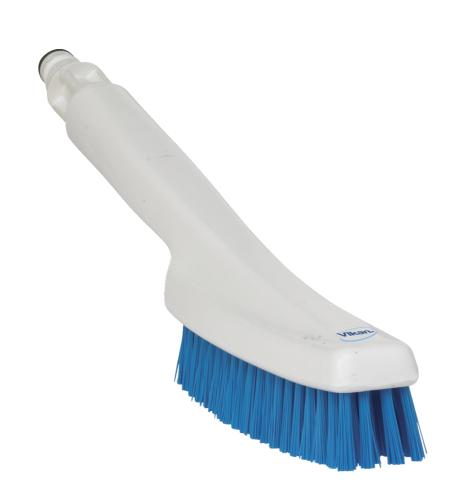
This waterfed hand brush is used for boot washing. The water runs through the centre of the brush and out through holes in between the bristles. Not suitable for use as a scrubbing brush as high volumes of water are consumed. The plastic coupling is suitable for standard coupling systems.
